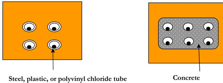
Figure 6A: Example of Draw-in Conduit System
